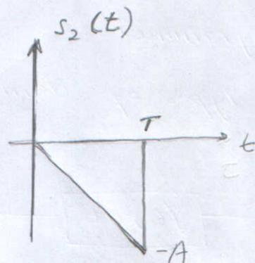
Solution: Since one orthogonal basis function is sufficient to represent both  $s_1(t)$  and  $s_2(t)$ , the given signals constitute ASK, thus one dimensional, that is
