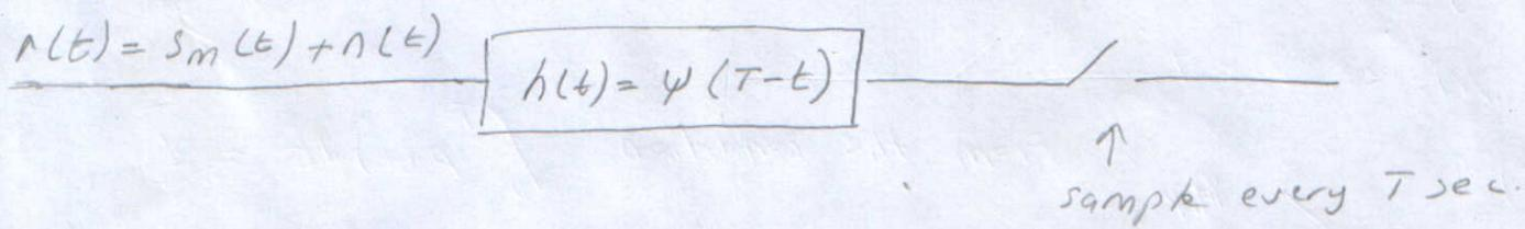
Output of MP detector [if  $s_1(t)$  is transmitted]
